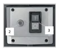
Switch on = Press Green [I] Button Switch off = Press Red [0] Button
