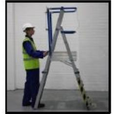
1. To commence deployment, place a foot on the bottom rung at the rear of the platform. Pull firmly down on the platform, until the deck is horizontal and the platform hooks are engaged.
