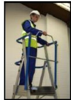
4. To increase the height of the platform, support the inner ladder whilst releasing both side locks by pulling them outwards. Raise the inner ladder until the required platform height is achieved and replace both side locks, ensuring they are fully engaged.
