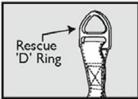
If the harness has an integral overhead rescue attachment, it must not be used for fall arrest, other than in conjunction with a retractable type fall arrester to BSEN 360 anchored above the user. The attachment should be either folded and stored in the Velcro pocket in the waist coat versions or attached with the Velcro loop to the chest strap at the back. The attachment must always be behind the head, never in front.
