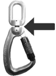
Check the safety hook, its gate locking function, and that the fall indicator has not activated (if present). If activated, the pin that connects the swivel eye and the hook (highlighted in the image by the arrow) will show red.
