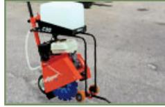
The Clipper C50 is a compact floor saw designed to carry out repairs to pavements and highway damage.
