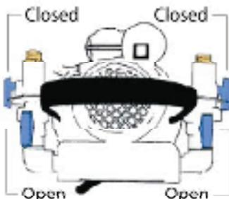
Position of pump valves during normal operation with full circulation through heating system – both isolating valves open, and dump valves closed.
