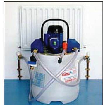
This is likely to be the least effective method due to the restrictive effect that valves (particularly thermostatic) may have on the flow rate.
