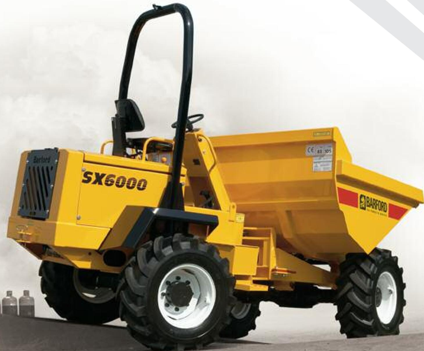
All Barford Dumpers come fitted with ROPs safety frames in a straight or folding configuration as required
