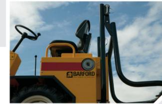
Over 1.59 metre reach allows for high discharge of up to 1 tonne into skips and small lorries
