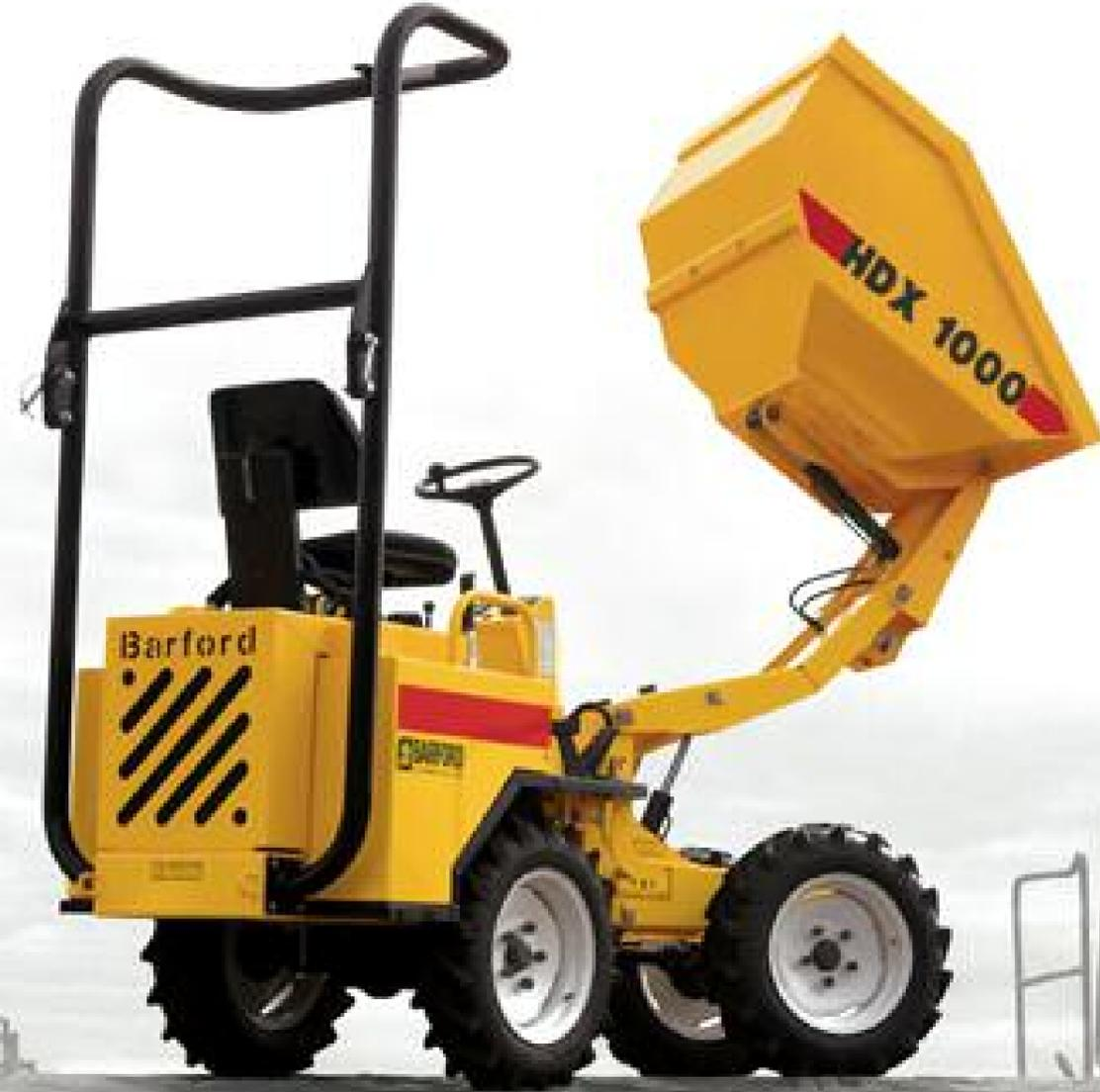
Fully certified ROPS folding safety frame allows for safe overnight container storage
