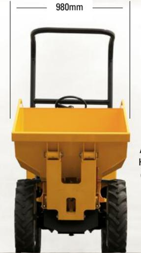
At just 980mm wide HDX can fit through even the tightest of spots with ease
