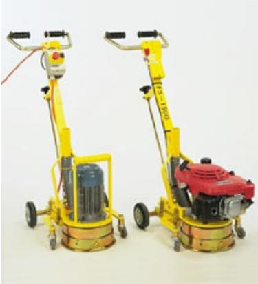
**Applications:** for concrete floors surface preparation, paint removal levelling, smoothing, light duty grinding removal light glue and mastics cleaning, keying
