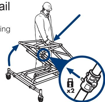
**IMPORTANT: Never** use the work station while the platform is in the lowered position.
