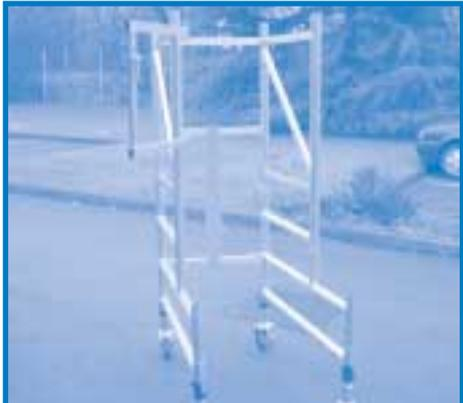
2. Stand the folding frame unit upright and push the two end frames apart so that the hinged bracing member is fully extended and the frame forms three sides of a rectangle when viewed from above and clip the front guard rail into place using the spring loaded pin.
