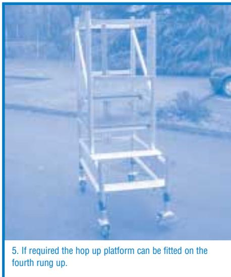
5. If required the hop up platform can be fitted on the fourth rung up.
