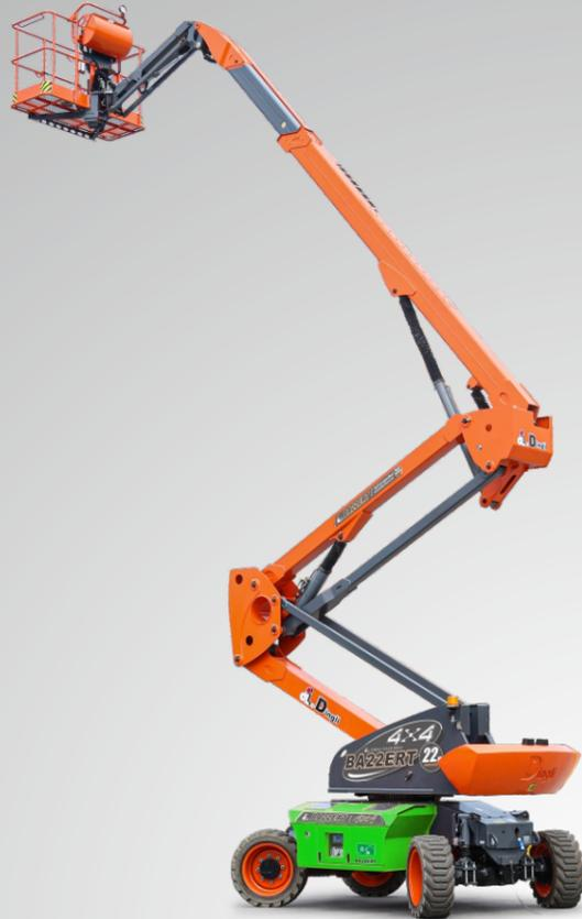
**Self-propelled Articulating Boom Lifts(Electric Axle Types)**
